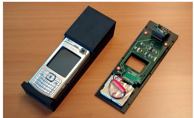
Figure 14. Prototype device with compass/tilt sensor.
